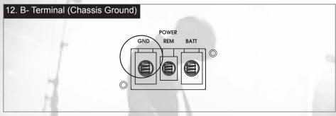
To avoid unwanted ignition noise caused by ground loops, it is essential that the amplifier be grounded to a clean, bare, metal of the vehicle's chassis. This metal surface should be solid, strong and connected directly to the frame of the car.
